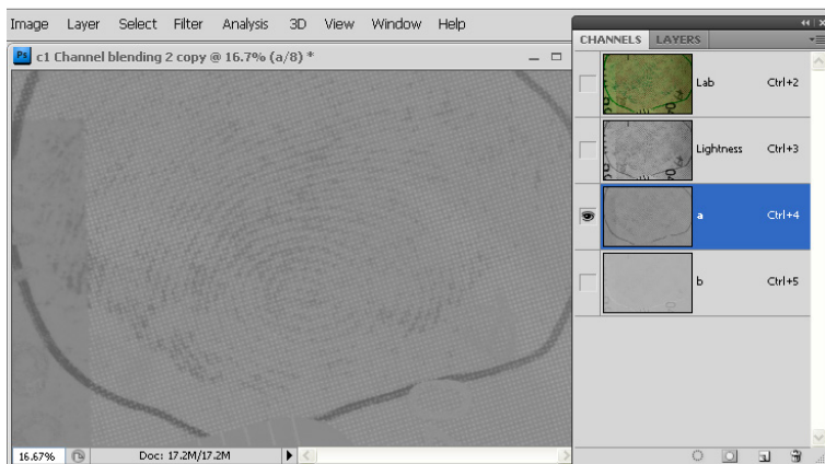
Figure 6 The “A” channel in Lab. Invert the “A” channel so that the ridges are dark, not white.
